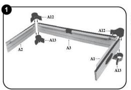
Attach long side (A3) and 2 small sides (A1&A2) in a horizontal position with large (A13) and small (A12) corner pleces, making sure the grooves in the rails line up correctly as shown above in Diagram 1.
