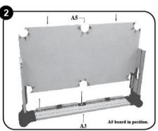
Slide board (A5) into upper grooves, closest to the bumpers, as shown above in Diagram 2. Make sure the felt side is facing towards the top of the games table.
